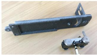
11. To mount the power truck, remove the gear retainer, part 1254, part and the wheel/axle assemblies from the power truck.
