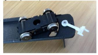
If wired for 2 Rail DC, the entire motorized floor assembly is now ready to begin test runs. From test experience, we have found that adding up to one ounce of weight under the A-Floor and one-half ounce under the 'B' floor provides the best operation
