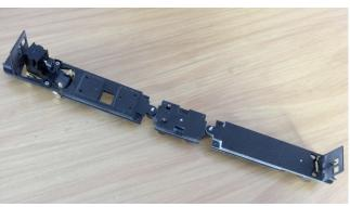
Note 4: You can wire your model in several ways, with or without provisions for overhead wire operation and, for DC or DCC. The 'A'-floor also has a provision for a 3 position DIP switch, a rectangular hole under the motor.
