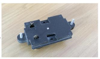
10. Attach the second trailing truck under the 'B'-floor with another screw M2x5 . Tighten the screw but allow enough play for the truck to swivel freely in all directions.
