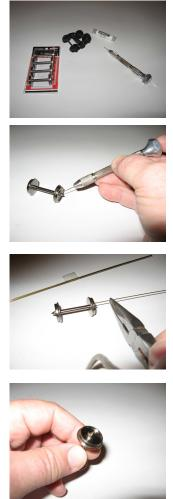
1. To remove and replace wheels from the truck, twist the sideframes and carefully extract or insert the wheelsets without damaging the axle point or the surface it revolves in. Do it carefully and the truck springs will not pop out. (An Athearn O-scale archbar truck is shown. Its plastic wheels will be replaced with metal Intermountain wheelsets. With Atlas O trucks, you must unscrew the sideframes and bolsters.)
