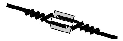
The wires will be looped together through each other with the plastic keeping them separated. When pulled they **compress** the plastic instead of stretching and breaking it.
