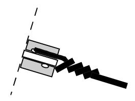
Feed the end of the second wire through the other hole and twist together over the opposite end.
