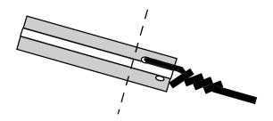
Drill the first one about 1/32 from one end and the second about 1/32 from the first. They should be close but there must still be plastic between the holes. When you feed the wire through the holes they must not touch. Cut the plastic just past the wire.
